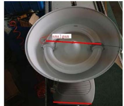
The bulb should be aligned with the amalgam caps and magnets facing east/west (right/left) and not up and down.
